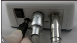
STEP4 : Illustration for connecting AC adapter Insert the AC adapter plug into the AC adapter connector, after hearing clicking sound as shown in Fig. 7.
