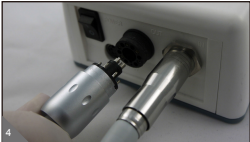
STEP3 : Illustration for connecting motor cord and control box Be sure there is no air or water coming from turbine hose when connecting. Fit the motor cord plug of the delivery unit to the motor connector piping and insert firmly. Rotate in counterclockwise direction. After hearing clicking sound, screw the nut properly with suitable force in clockwise direction completely, shown as Fig.5.
