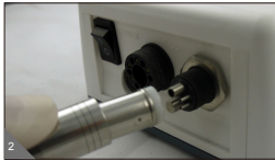
STEP2 : Illustration for connecting turbine hose connector Be sure there is no air or water coming from turbine hose when connecting. Fit the turbine hose plug of the delivery unit to the turbine hose connector piping and tighten completely. Rotate in counterclockwise direction. After hearing clicking sound, screw the nut properly with suitable force in clockwise direction, shown as Fig.3.
